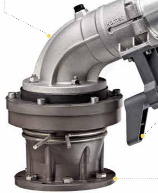
Flange: External Ø 168 mm (6 39/64"), 6 holes Ø 10.5 mm (13/32") on pitch circle
