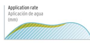
Schematic water distribution profile **without** dynamic jet-breaker
