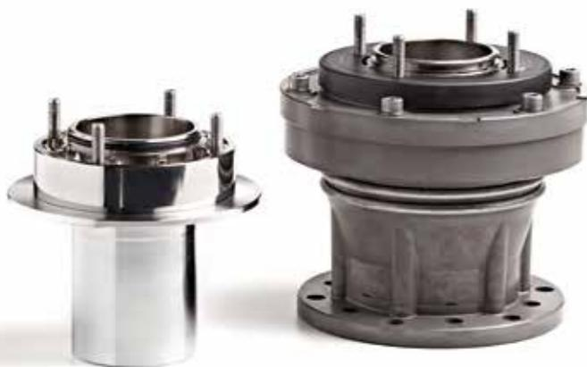
The Automatic Brake System is unique in its function due to the materials used. The internal parts are made of chemically treated stainless steel and inserted into an anodized aluminium housing to increase the resistance to corrosion and wear.
