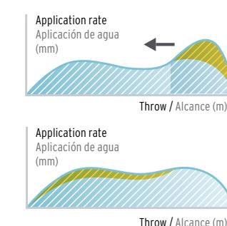
Schematic water distribution profile **without** dynamic jet-breaker
