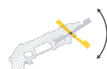
The **Komet Balance System** is based on the interaction between the self-adjusting brake and deflector. The resulting balanced operating mode allows for an excellent performance at all pressure and flow levels. The interactive balancing between the two elements is continuous and automatic.
