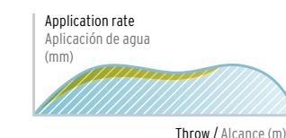
Schematic water distribution profile **with** dynamic jet-breaker
