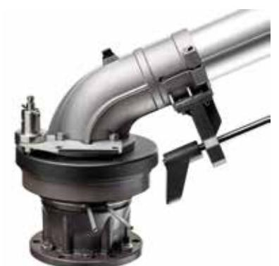
Easily installed on top of the big volume gun base, the two different settings of the Komet Transport Lock either permit or prevent the big volume gun from turning. This way it can remain installed also during operation.
