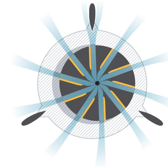
The even number of streams and odd number of specially designed body legs means that only one stream hits a body leg at any given time.
