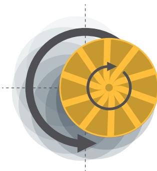
The deflector rotates around the central sprinkler axis as well as its own inclined axis.
