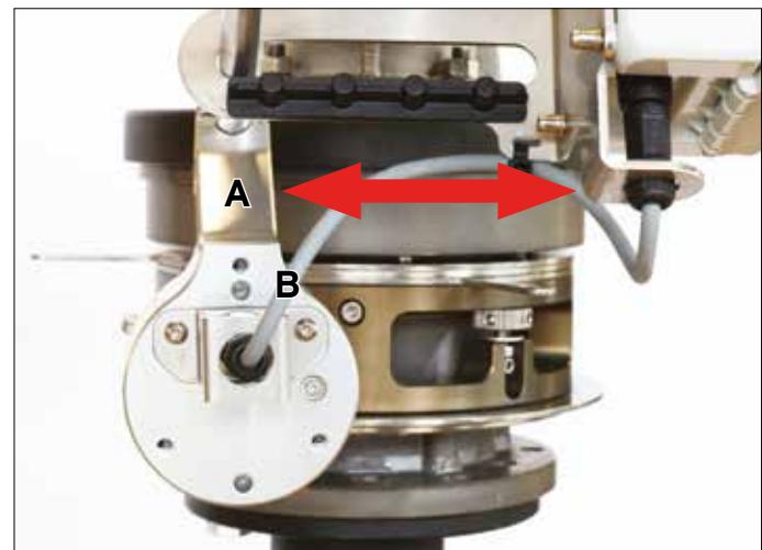
Move the inverter circuit from left to right (A), make sure that cable (B) does not get under tension.
