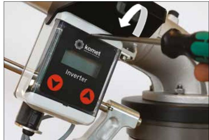
Unlock the lid of the timer with a flat screwdriver by **TURNING** the screwdriver, then remove the lid.
