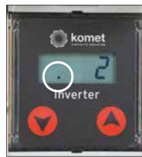
**ATTENTION! The timer is very sensitive.** Before leaving the irrigation cart, make sure that the timer is activated but has not yet started the countdown.
