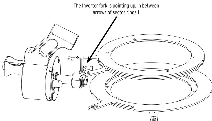
After the preset time has elapsed, a magnet is released, unlocking the inverter fork and bringing it into **search position**.
