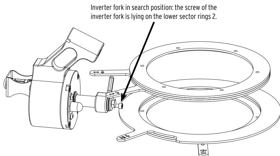
The inverter fork in search position is now moving along the lower sector rings, until the screw is falling through the gap and the inverter fork is locked in its **lower position**. The gun is now operating in sector 2.
