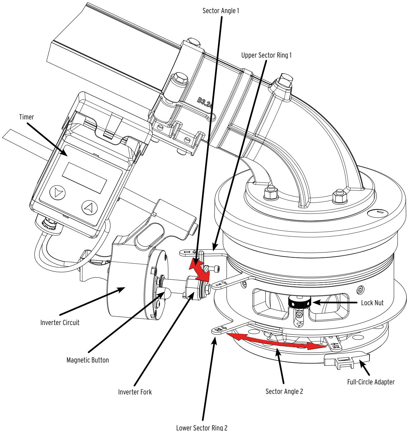
The patented Komet Inverter allows to operate the gun in two completely independent sector angles. Starting in sector 1, the gun turns automatically into sector 2 after a preset time has elapsed. The required time will be set through a timer.
