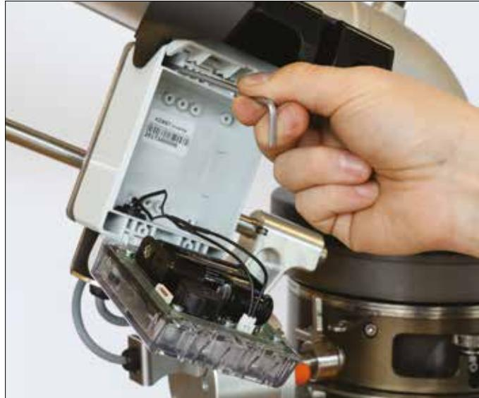
Install the timer with the 4 supplied Allen screws (M4 x 12). Make sure that the plug is facing downwards.
