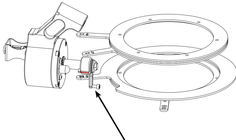
The Inverter fork is falling through the gap of the sector rings 2.
