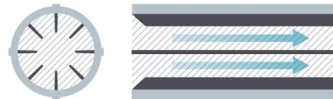
The Komet Twin Barrel is designed to allow the water to reach the nozzle with the least possible turbulences and pressure losses
